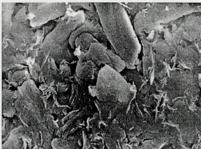
Fig. 5. SEM photo demonstrating the upper surface of a tablet prepared from nitrazepam and A101.
