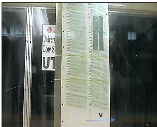
a) Tuft Test at V = 10 m/s Angle of Attack 0^\circ
