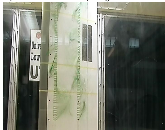
e) Tuft Test at V = 30 m/s Angle of Attack 16^\circ
