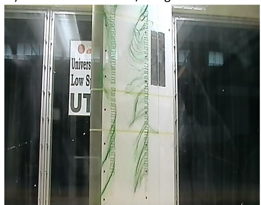
f) Reversed flow condition during tuft testing
