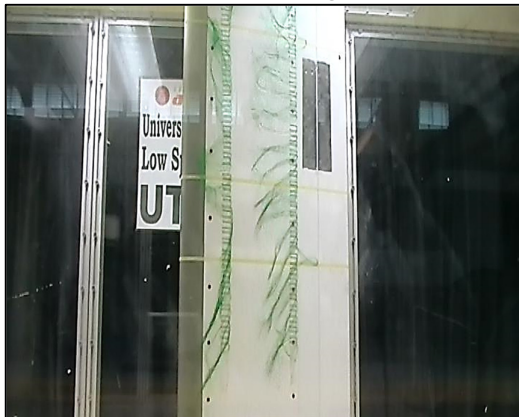
c) Tuft Test at V = 10 m/s Angle of Attack 14^\circ
