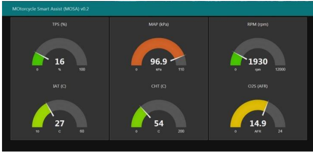
Figure 9. Dashboard UI nodes rendered web-based GUI shows 6 gauges represents readings of different kinds of sensors
