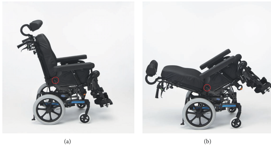
FIGURE 1: Wheelchair “Rea Dahlia 45” (Invacare®) in the upright reference posture (a) and the maximum tilted/reclined position (b). The pivot point of the backrest is highlighted by a red circle.
