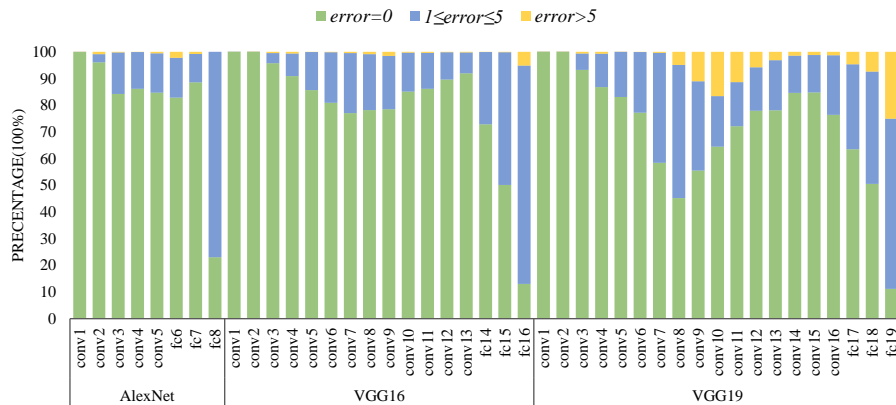
Fig. 4. Error distribution across the neural network layers when highest BER is used in AlexNet, VGG16 and VGG19.
