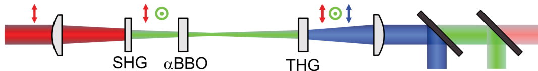
Fig. 6.8: THG scheme with delay compensation: SHG: in a 0.8 mm, type I BBO cut at 23.5°; \alpha BBO: delay compensator, 1.1 mm thick \alpha BBO cut at 70.0°, THG: in a 1.0 mm, type II BBO cut at 40.0°.
