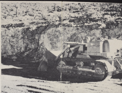
TEXAS TALC CO.'S surface outcrop is broken and loaded by a bulldozer mounted single tooth ripper and front loader.
