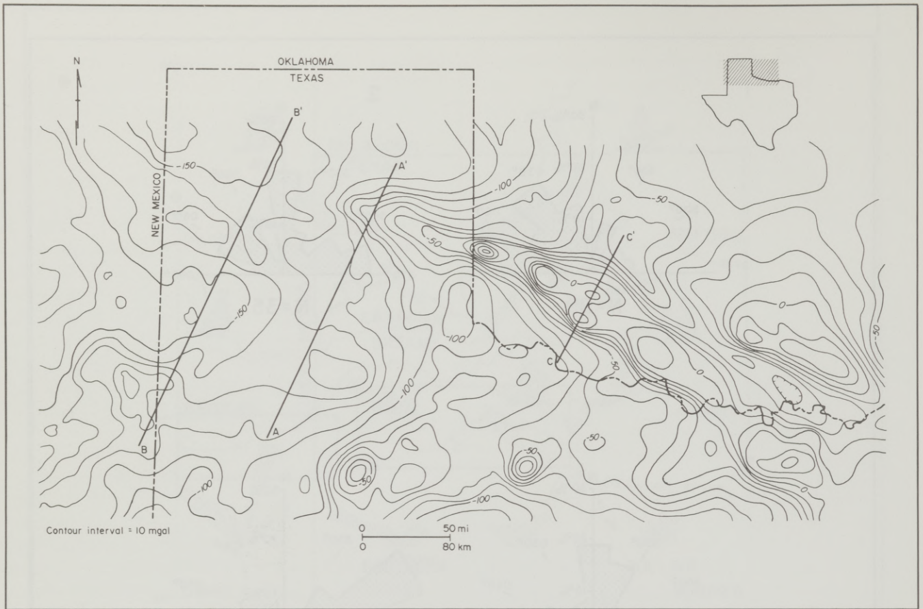
Figure 41. Simple Bouguer gravity anomaly map, Texas Panhandle and vicinity. See 2-milligal contour map (pl. VI). A-A' and B-B' are locations of gravity models discussed in this report (see figs. 43 and 44).
