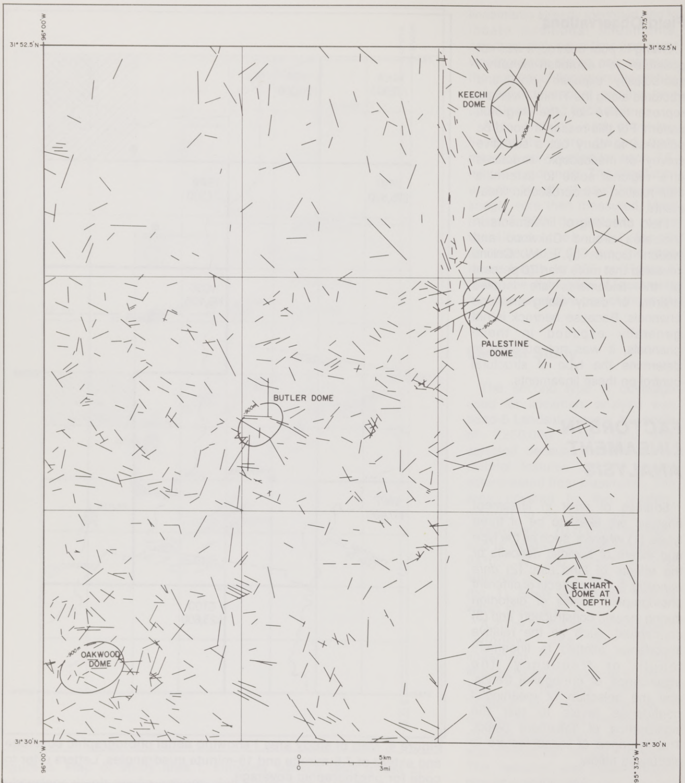
Figure 5. Map of southern part of study area I showing relation between airphoto lineament pattern and salt domes.
