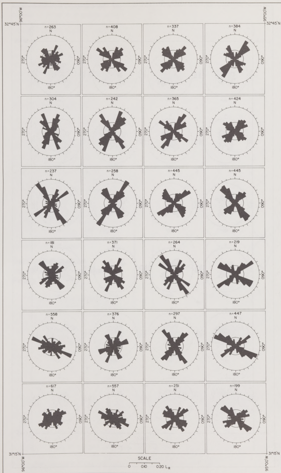
Figure 13. Polar graphs showing relative lengths ( L_R ) of lineaments in each 15-minute quadrangle in study area I. Inner circle represents arithmetic mean.
