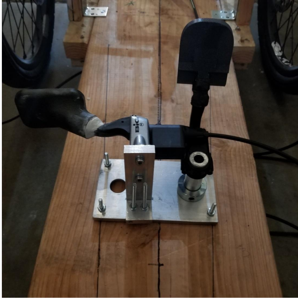
Figure 35 Final brake pedal mount assembly. Front brake pedal (left) and rear brake pedal (right).
