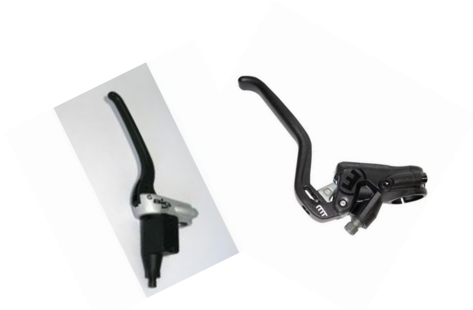
Figure 22 The Magura Big Twin brake (left) has a vertically oriented master cylinder, whereas the Magura MT4 brake (right) has a horizontally oriented master cylinder.
