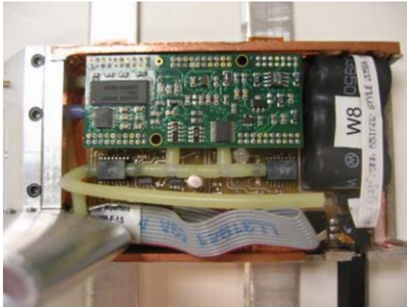
Figure 1-1: BLDS with cover removed to show internal circuitry (Westphal et al. 2008).
