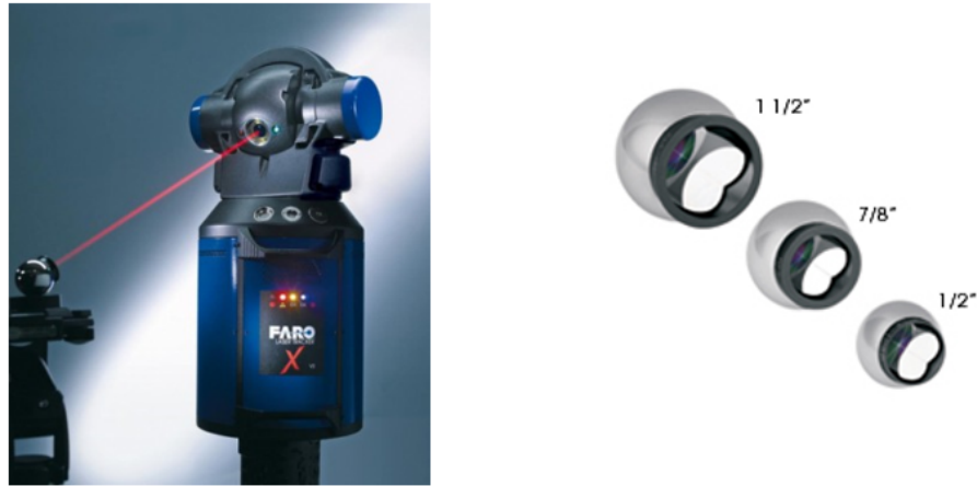
Figure 7.2: FARO laser tracker (left) and its corresponding SMR targets (right).
