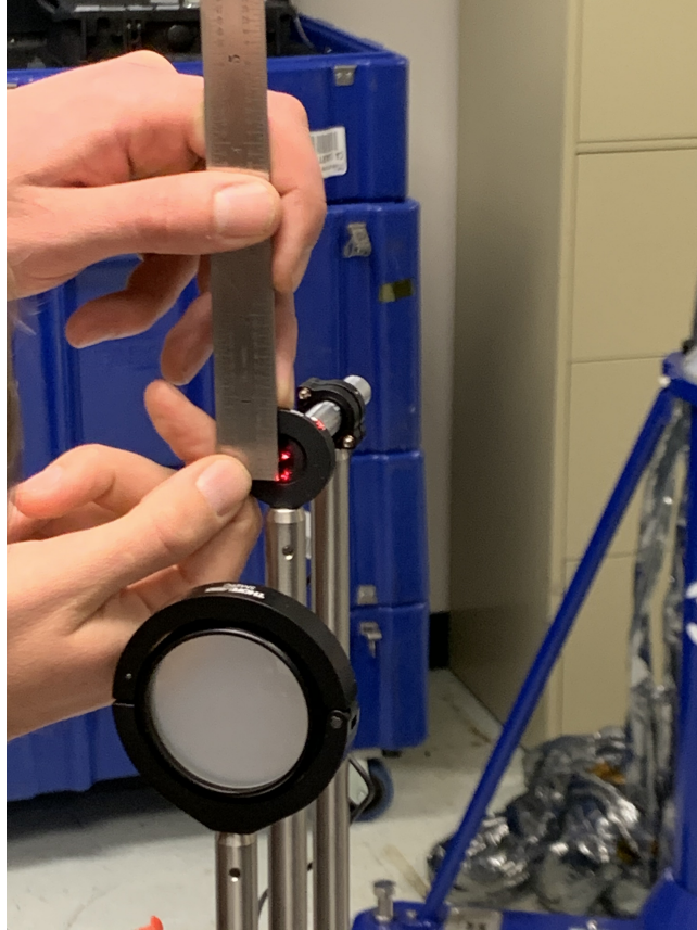
Figure 9.9: Measurement of the reflected spot during the alignment process for the top mirror. The measurement was used to calculate the required tip/tilt adjustment of the mirror stage.
