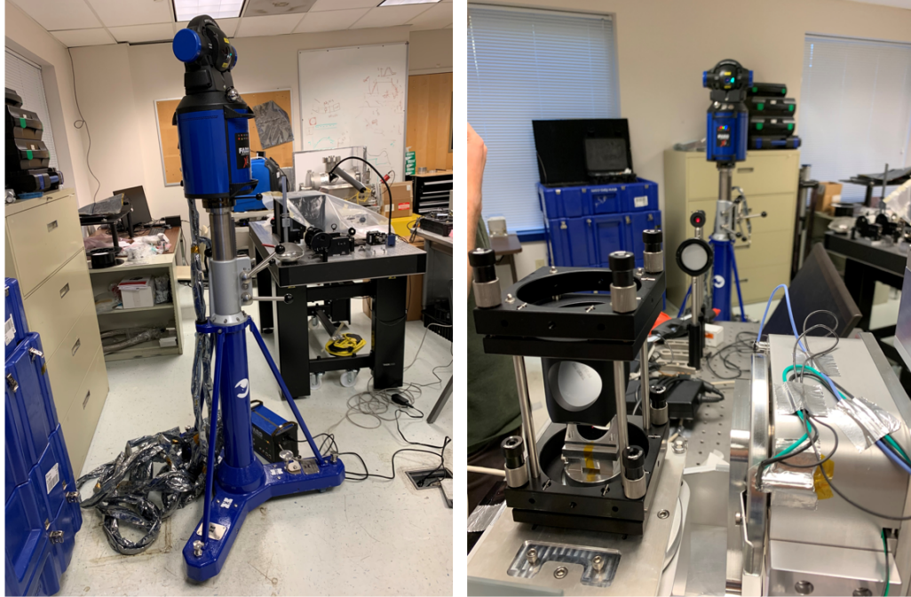
Figure 9.6: Image of the FARO laser tracker (left) and a view of the optical GSE with the laser tracker in the background (right).
