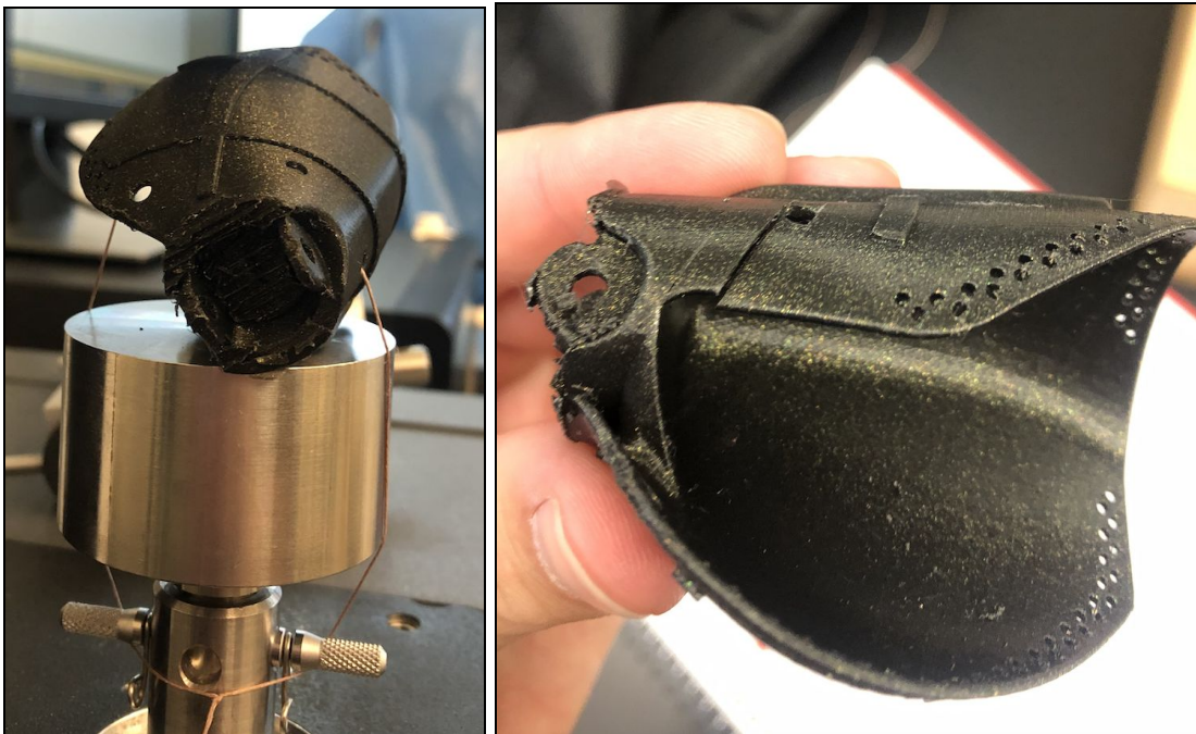
Figure 38 & 39. Proximal compression testing 02/20/20, orientation 2, attempt 3.
