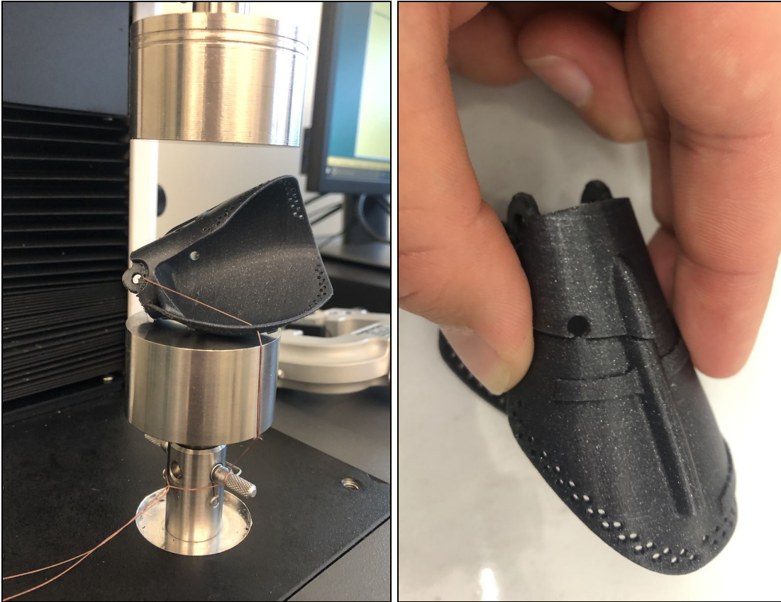
Figure 28 & 29. Proximal compression testing 02/20/20, orientation 1, attempt 1.
