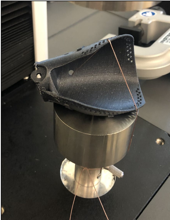
Figure 32 & 33. Proximal compression testing 02/20/20, orientation 1, attempt 3.
