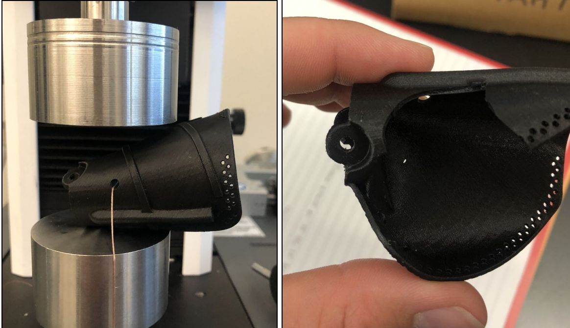
Figure 36 & 37. Proximal compression testing 02/20/20, orientation 2, attempt 2.
