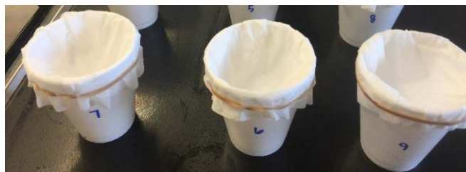
FIGURE 4-2: Put the coffee filter over the cup so that it is loose/dips into the cup. Place the rubber band around the filter/cup so that it stays when you pour the coffee through. Remember to label your cups as instructed, and include the usual sample label information (i.e., "Coffee 100C, Your initials, today's date")
