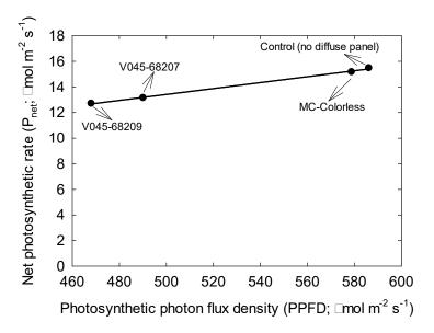
Canopy light use efficiency, the ratio of  $P_{net}$  to incident PPFD, increased slightly by 2 to 3% under diffuse panels V045-68207 and V045-68209.
