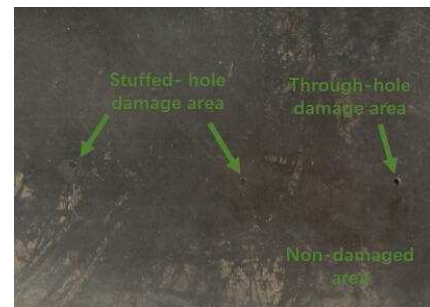
FIGURE 12. The material with artificial damage.
