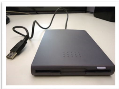
Figure 3: External USB floppy disk drive
