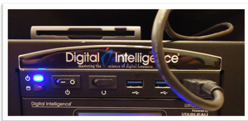
Figure 4: External USB floppy plugged into FRED USB port
