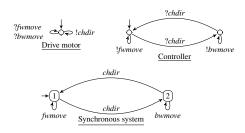
Figure 1: An illustration showing the impossibility of establishing the diamond property in certain synchronous systems.
