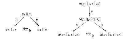
Figure 4: An illustration showing that nondeterministic reception of messages u in a desynchronisable synchronous system leads to branching bisimilar states  $p_2 || s_2, p_3 || s_2$ .
