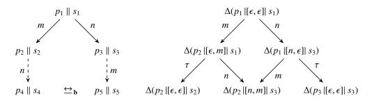
Figure 6: An illustration showing that the communication of two send messages m, n by different processes can be done in any order in a desynchronisable synchronous system.
