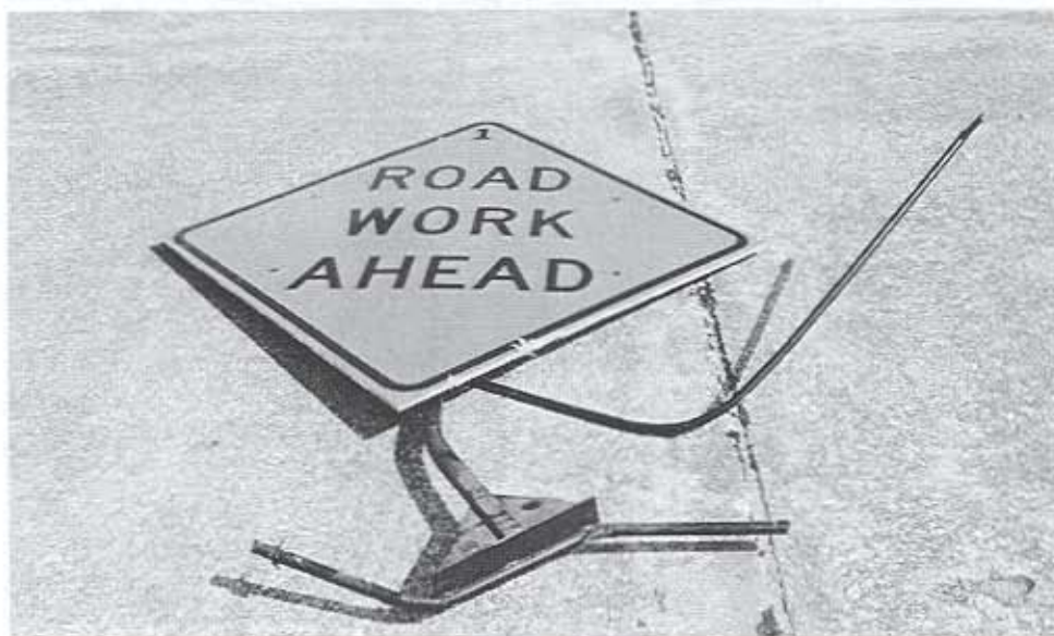
Figure 15. System No. 1 Damage, Test I-1
