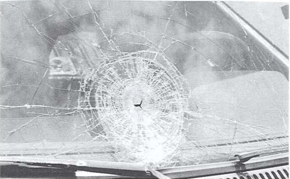
Figure 17. Vehicle and Windshield Damage, Test I-1
