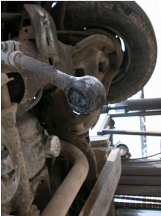
Figure 33. Vehicle Undercarriage Damage, Test KTB-1
