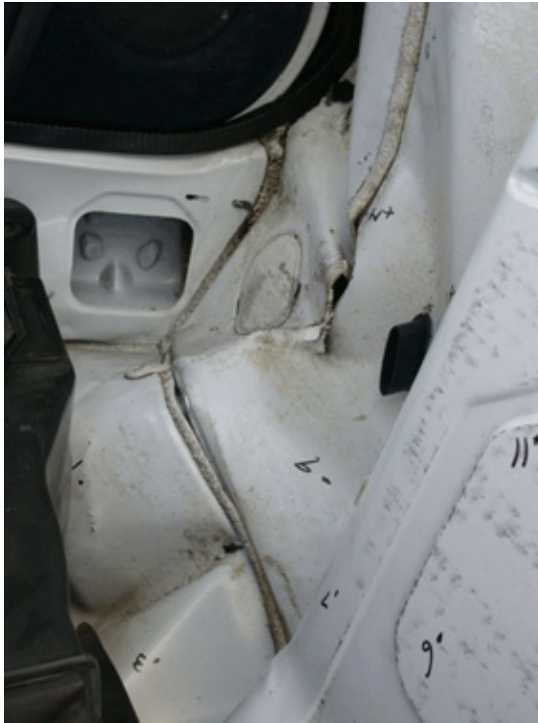
Figure 34. Occupant Compartment Damage, Test KTB-1
