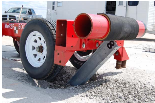
Figure 1. Impacted Post Contacting Backslope of Testing Pit
