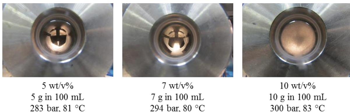
Figure 2. View cell solubility tests for rac -LA in scCO 2 . The first two conditions show complete solubility but there is only partial solubility at 10 wt/v% (right)
