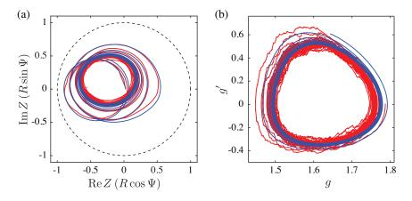
Figure 1. Validation of mean field reduction. Comparison of dynamics for mean field model (blue) (2)–(4) and simulation of 500 coupled QIF neurons (red) (7). (a) Phase plane of the Kuramoto order parameter  $Z = Re^{i\Psi}$ . (b) Synaptic conductance g vs rate of change of synaptic conductance g'. Parameter values:  $\eta_0 = 20$ ,  $\Delta = 0.5$ ,  $v_{\text{syn}} = -10$ ,  $\kappa = 1$ ,  $\alpha = 0.95$ .
