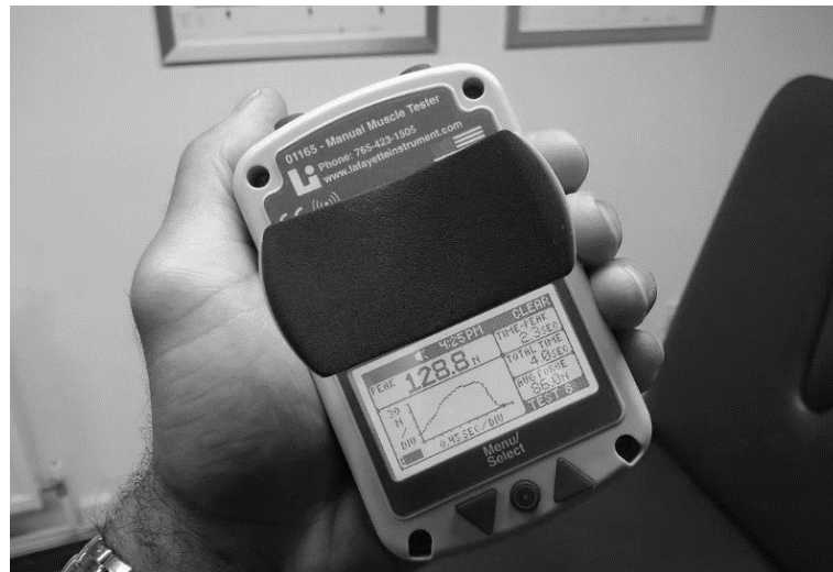
Figure 32 - Lafayette Manual Muscle Tester (LIC.01163, Lafayette Instrument Company, Loughborough, Leics, UK
