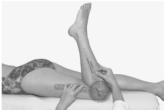
Figure 24 – Quadriceps test position showing a PDT-Com score 3 (70-79°) as measured using a universal goniometer
