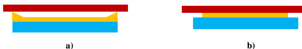
Fig. 5.14. The gap between the mask and the photoresist a) with edge bead; b) without edge bead
