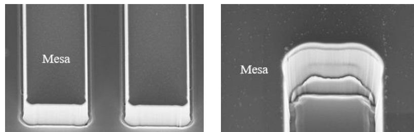
Fig 4.9. Dry etching results with 50sccm SF 6 , 0sccm Ar and 40mT pressure
