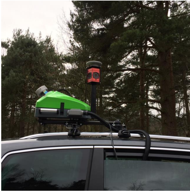
1 2 3 4 5 6 7 8 9 10 11 12 13 14 15 16 17 18 19 20 21 Figure 6(b): StreetMapper MLS system (the camera system in the picture was not used in 22 this particular test) 23
