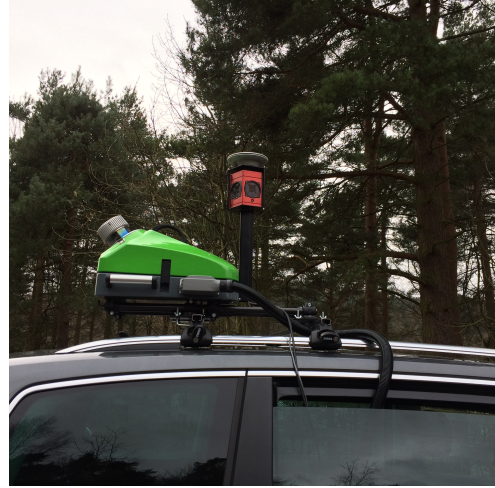
(b) StreetMapper MLS system (the camera system in the picture was not used in this particular test)
