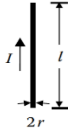
Figure 3.1: Inductance for a straight wire with length l and diameter of 2r , is calculated by L=200l (\ln (2l/r)-1) \times 10^{-19} [79]
