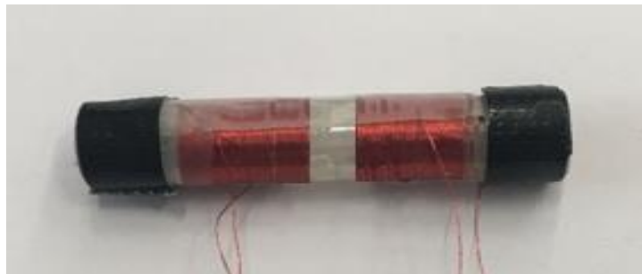
Figure 6.46: The preferred geometry of the coil for the cylindrical sensor from the models (a), and constructed cylindrical air cored sensor (b)
