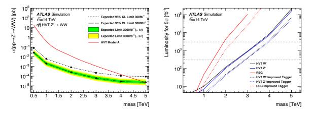
Fig. 6.4.8: Left: 95% C.L. upper limit for the HVT Z' via  $ggF/q\bar{q}$  production. Right: expected luminosity required to observe a  $5\sigma$  signal significance for the HVT W' (black), HVT Z' (blue) and  $G_{RS}$  (red). The solid curves shows the sensitivity using the current W/Z-tagger and the dashed curves for a future tagger that has a 50% increased signal efficiency and a factor two increased rejection of background.
