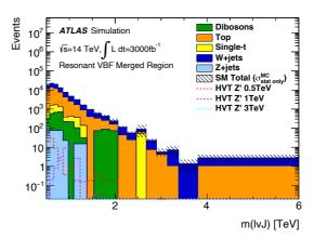
Fig. 6.4.7: Left: final  $m(\ell\nu J)$  distribution in the merged signal region for the  ${\rm ggF/q\bar q}$  search. Right: final  $m(\ell\nu J)$  distributions in the merged signal region for the VBF search. Background distributions are separated into production type. HVT signals are superimposed as dashed curves where appropriate.
