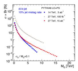
**Fig. 6.4.4:** Expected 95% C.L. upper limits obtained from the  $M_{jj}$  distribution for jets identified as b-jets. The limits are set on fiducial cross-section times the BR to two jets for a hypothetical BSM signal approximated by a Gaussian contribution to the dijet mass spectrum. The limits are obtained for the HL-LHC and HE-LHC energies.
