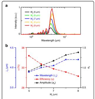
Fig. 5 Effects of the spot size of the input signal pulse on the output mid-IR pulses. a The spectra of the output infrared pulses under different spot radii of the signal pulse. b The central wavelength  $(\lambda_c)$ , normalized amplitude  $(a_{ir})$ , and energy conversion efficiency  $(\eta)$  of the mid-IR pulses as a function of the signal laser spot radius
