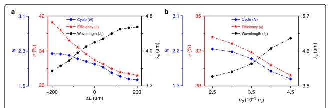
**Fig. 3 Effects of the plasma parameters on the output mid-IR pulse.** The mid-IR optical cycle number (*N*), energy conversion efficiency ( $\eta$ ) and central wavelength ( $\lambda_c$ ) evolution with changing **a** channel length  $L = \Delta L + L_0$  (with  $L_0 = 1597 \,\mu\text{m}$  and  $n_0 = 3.5 \times 10^{-3} n_c$ ) and **b** plasma density  $n_0$  (with fixed  $n_0 L = 5.59 \,\mu\text{m} \cdot n_c$ )
