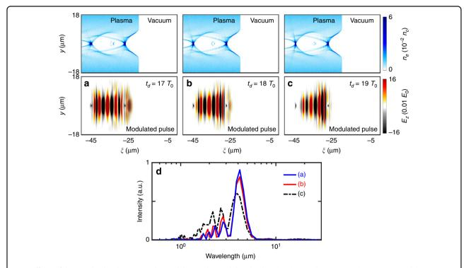
Fig. 6 Effects of the initial pulse duration and time delay on the modulated pulse. The electron density  $(n_e)$  in the upper row and the transverse electric field of the signal laser  $(E_z)$  in the lower row are shown for three different delay times  $t_d = 17T_0$  (a),  $18T_0$  (b) and  $19T_0$  (c). d The spectra of the modulated signal pulses
