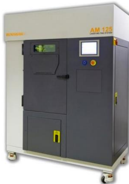
Figure 3-3 Renishaw AM125 Selective Laser Melting Machine (Renishaw SLM 2013)
