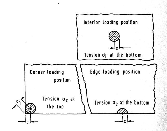
corner is not in complete contact with the subgrade due to upward warping of the slab. Spangler (9), after conducting large-scale indoor experimental tests, confirmed Kelley's formula for corner loading and suggested a simplification of the formula which yields substantially the same results.
