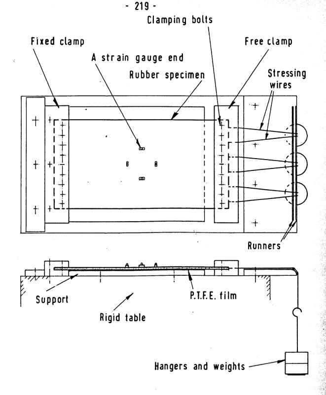
properties of a hard rubber is that the electrical strain gauges commercially available are many times stiffer than the rubber itself. Thus, the gauges would stiffen the test material at the points at which they were affixed. This would result in apparent properties which could be grossly incorrect.
