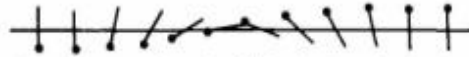
Figure 6.6: The Sine-Gordon soliton as an infinite line of interacting pegs, from Ryder [51]
