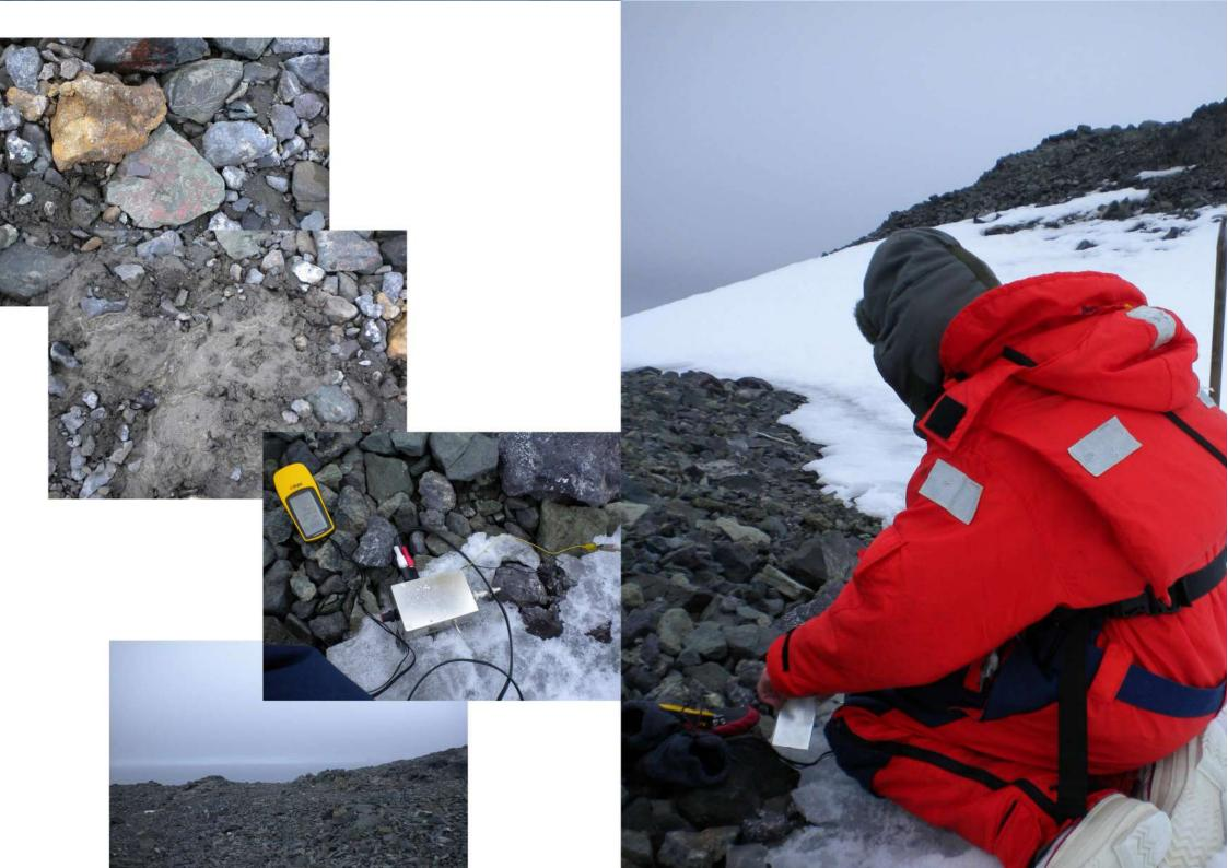
The hydrophone is a transducer device, similar to a piezo electric microphone that works transforming acoustic pressure into electrical impulses. The focus of this field work was to detect imperceptible signals, acknowledging the particularity of the terrain that is unpopulated and thus free from massive artificial electromagnetic very low frequency signals as well as wilderness presence and biodiversity that make it prone to detect otherwise unreachable animal populations.
