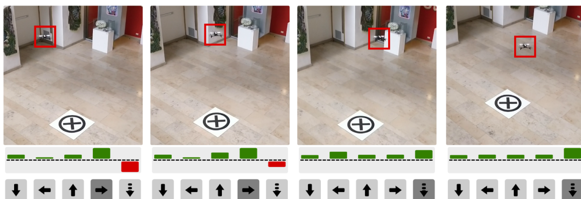
Figure 8. Snapshots of the descending phase with the utility distribution over all the actions. Descent has a negative utility (red bar) when the drone is not centred on the marker.
