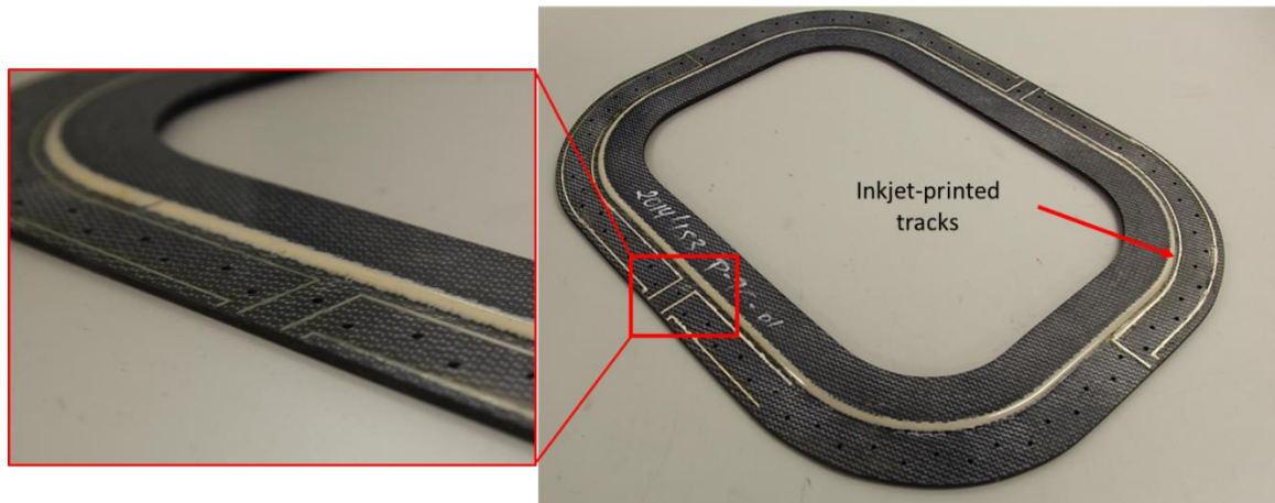
Figure 3 Inkjet printed tracks onto the window frame
