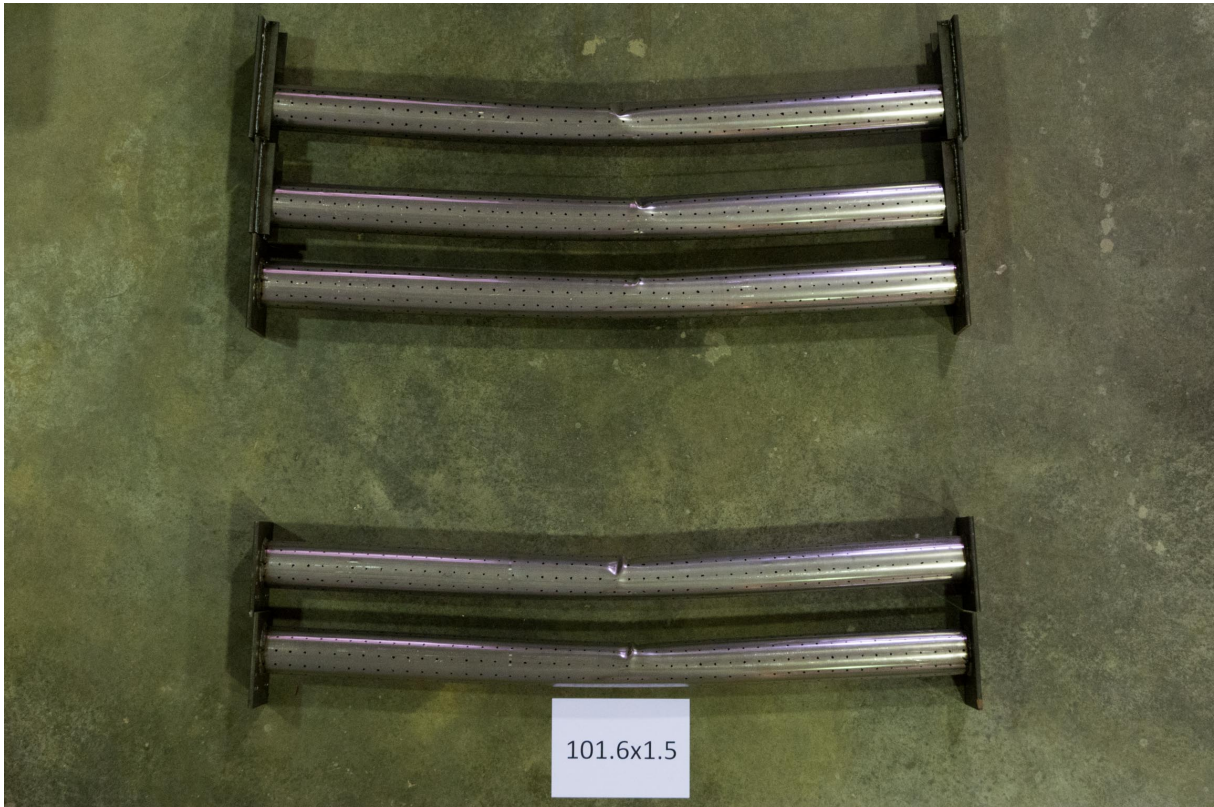
Figure 13: Deformed 101.6×1.5 CHS long beam-columns, with load eccentricity increasing from bottom to top.
