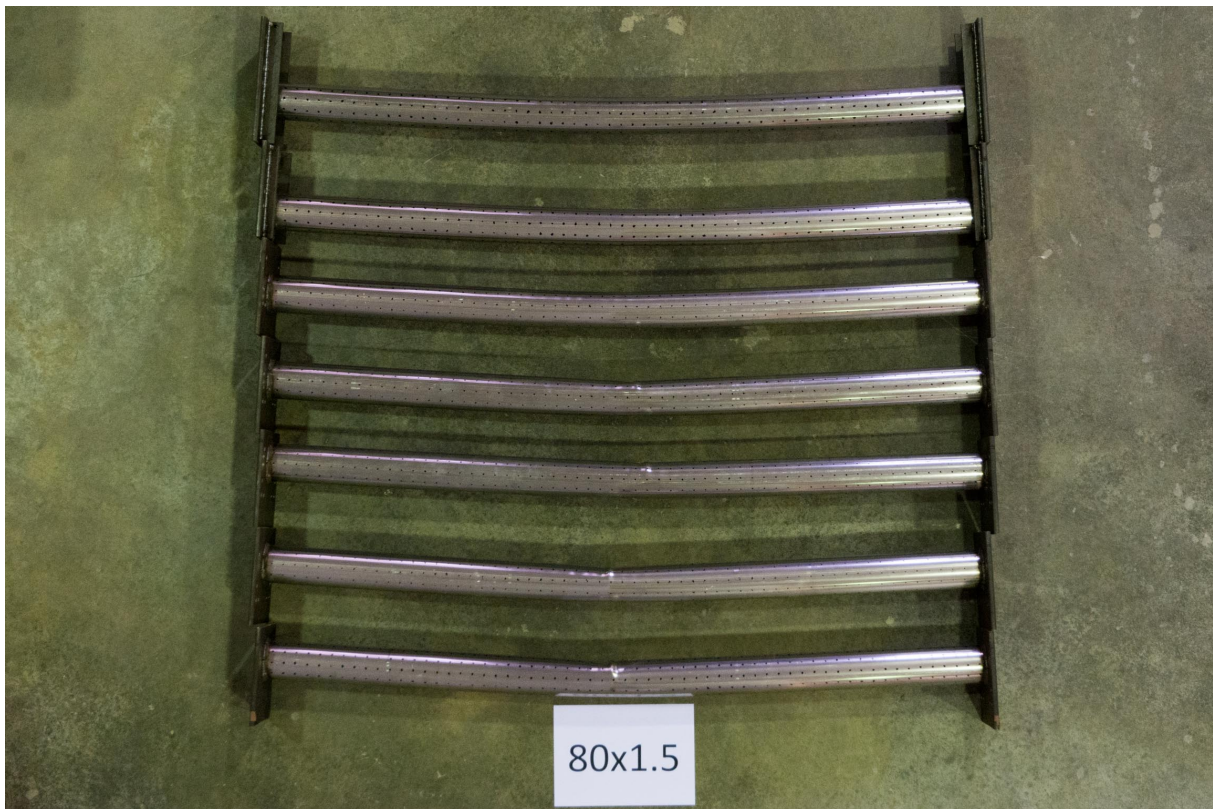
Figure 12: Deformed 80×1.5 CHS long beam-columns, with load eccentricity increasing from bottom to top.
