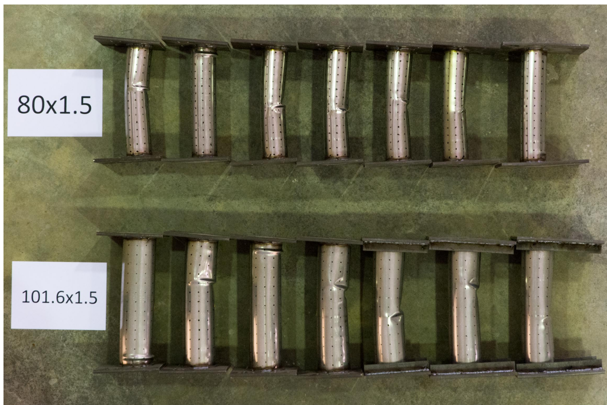
Figure 9: Deformed short beam-columns, with load eccentricity increasing from left to right.
