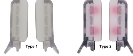
Fig. 6. Type 1 fingertips with only silicone pad and type 2 fingertips with pressurized air cavities
