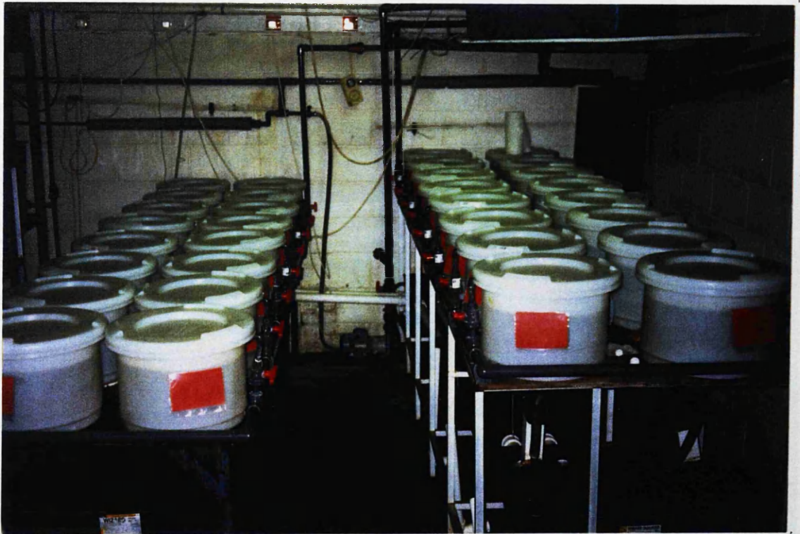
Plate 1 Experimental fingerling rearing recirculation system (as described in 3.1)
