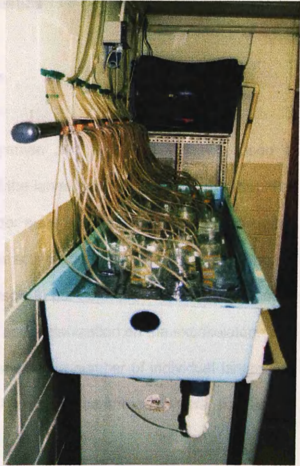
Plate 18. Air distribution to the LRC.
