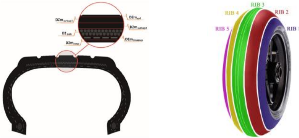
Figure 2. Example of thermoRIDE tire mesh configuration.
