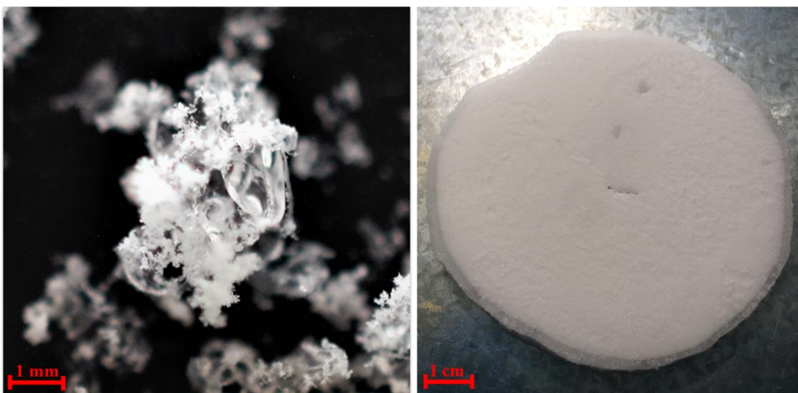
Figure 3.4.2. Left: water frost accumulating on a CO 2 ice grain. Right: a rim of water ice around a thin slice of carbon dioxide snow.
