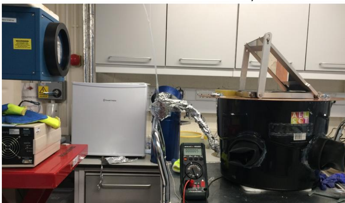
Figure 3.4.5. Schematic and photograph of final experimental set up which enabled temperatures to be reduced and moisture content within the chamber kept to a minimum.
