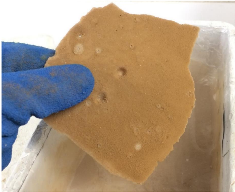
Figure 8.1.2. Once devoid of liquid nitrogen, the dusty snow mixture sintered rapidly, so that it became unusable for experimentation. This solid slab formed in less than a minute when left at ambient conditions.
