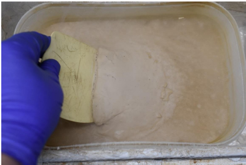
Figure 8.1.3. 0.1% Mars simulant dust mixed with CO 2 snow and suspended in liquid nitrogen.
