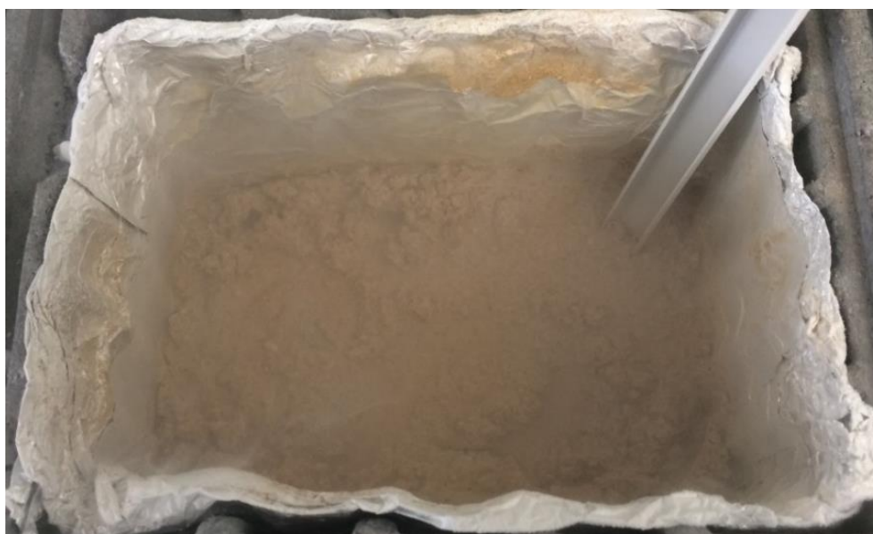
Figure 8.1.1. The mixture of 1% Mars simulant (<20 \mu\text{m} grain size) with CO 2 snow rapidly sintered, taking on a lumpy consistency if not fully submerged in liquid nitrogen. Note the dark colouring of the snow, despite just 1% dust content.
