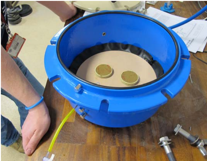
Figure 1 Pressure (extractor) plate apparatus (ceramic plate type) with lid removed showing two test specimens.
