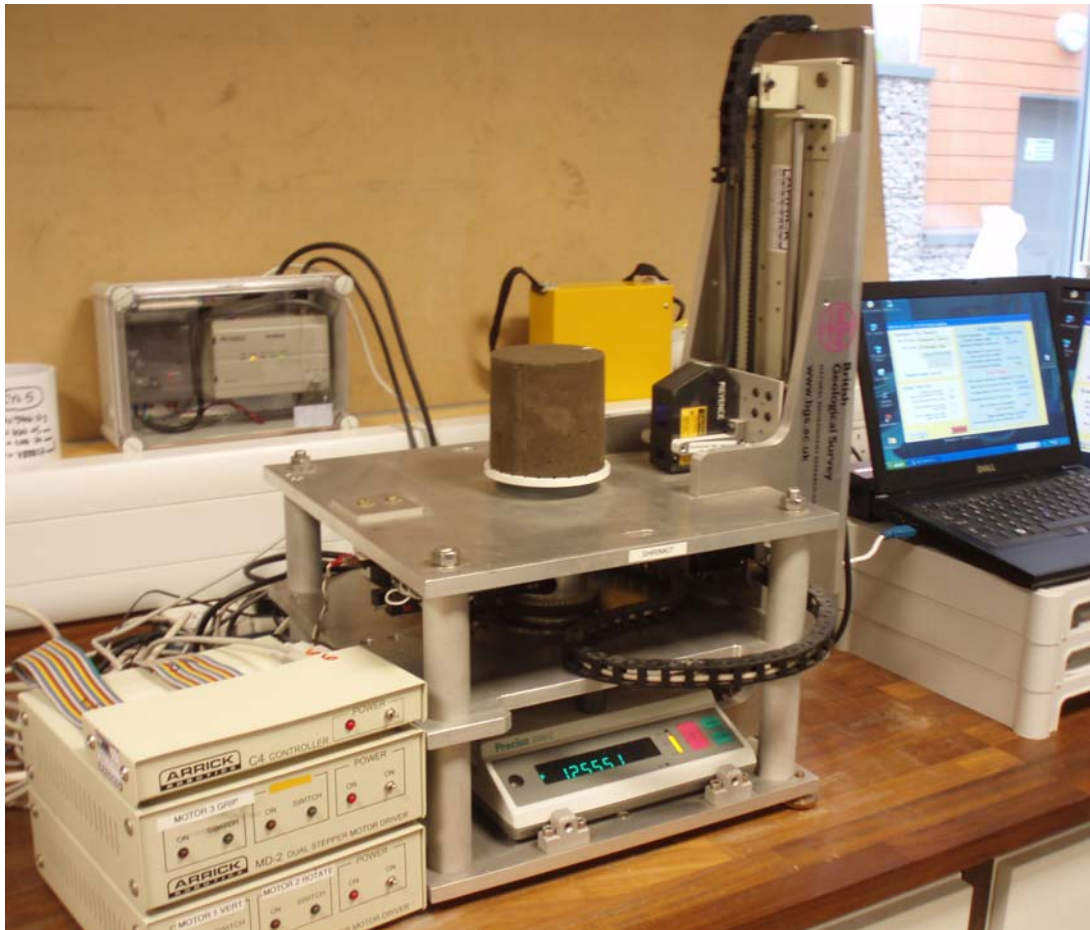
Figure 6 Shrinkage limit apparatus [version 2: fully automated, 'SHRINKiT'] 2012
