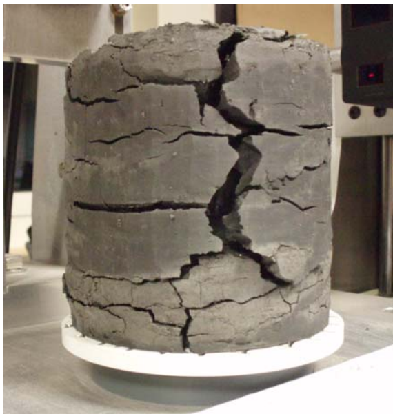
Figure 19 Image showing severe shrinkage cracks developed during a test on a specimen of ‘undisturbed’ Gault Formation (P83B) clay from a borehole at Niton (I.O.W.)
