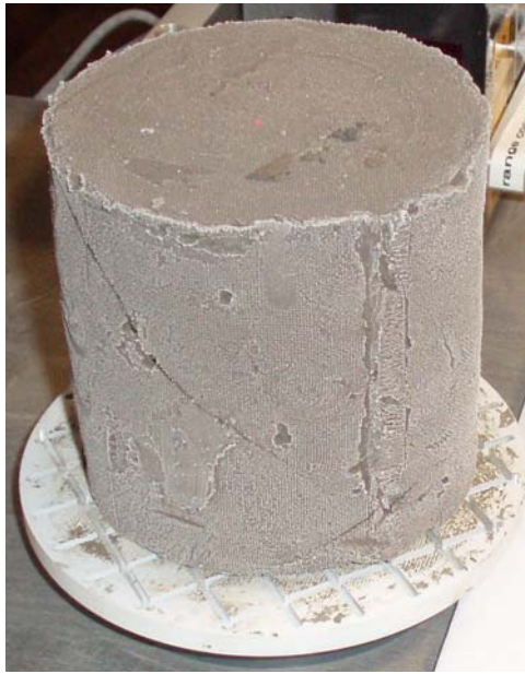
Figure 20 Image showing minor shrinkage cracks on a specimen of ‘remoulded’ London Clay Formation from Colchester Quarry, Essex.
