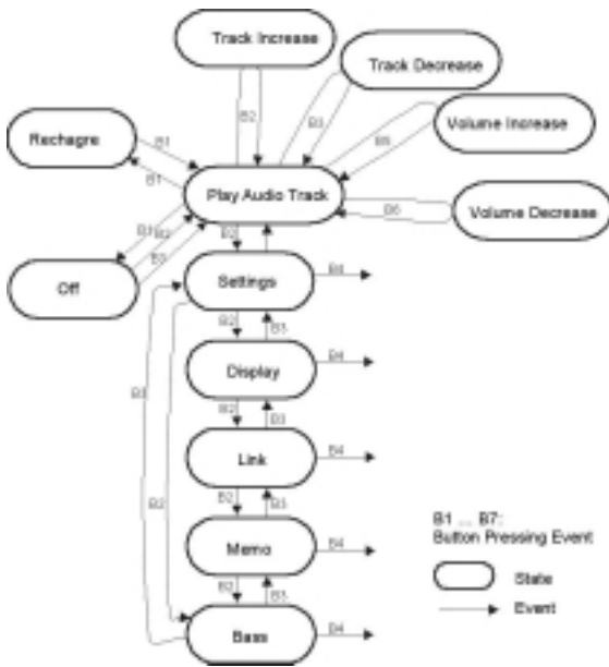
Figure 3 Sample State Diagram of MP3 player interface
