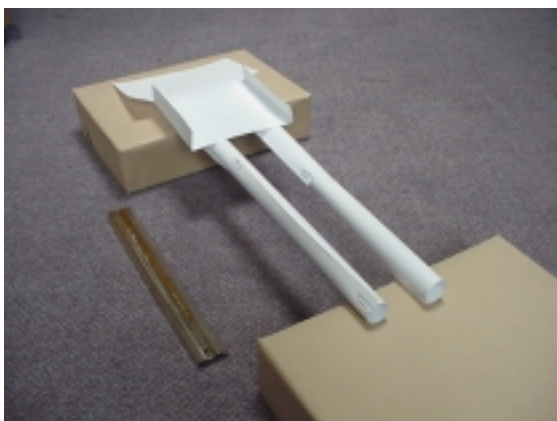
Figure 1 Example of tubular solution. Part of decking removed to show structural arrangement
