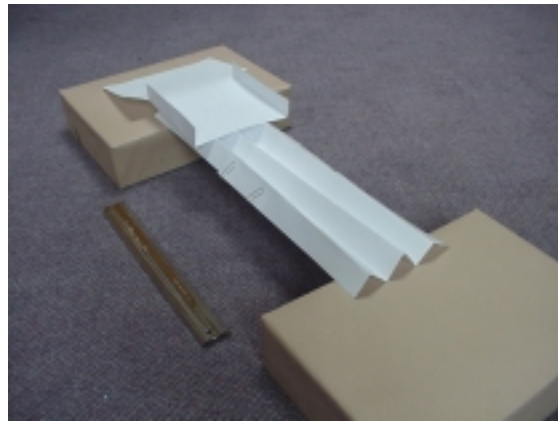
Figure 2 A “concertina solution”. Folds aligned with long axis of structure. Part of decking removed to show structural arrangement
