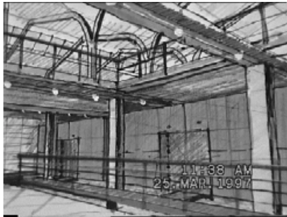
Figure 7 Perspective drawing produced by CAD, then hand rendered
