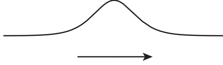
Fig. 1. A symmetric solitary wave of elevation is found for \alpha = \alpha_* - \delta , 0 < \delta \ll 1 ; it decays exponentially and monotonically to a horizontal laminar flow far up- and downstream.
