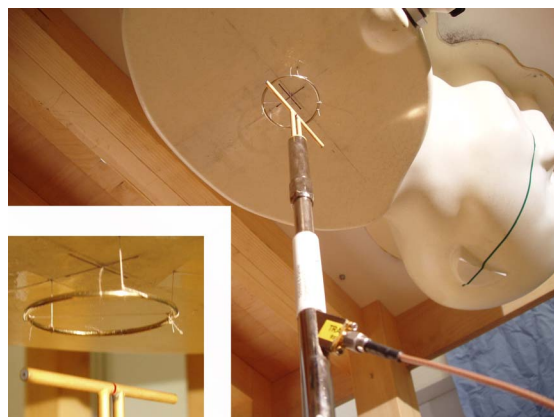
Figure 1. A circular ring and dipole positioned under the flat section of the SAM twin phantom.
