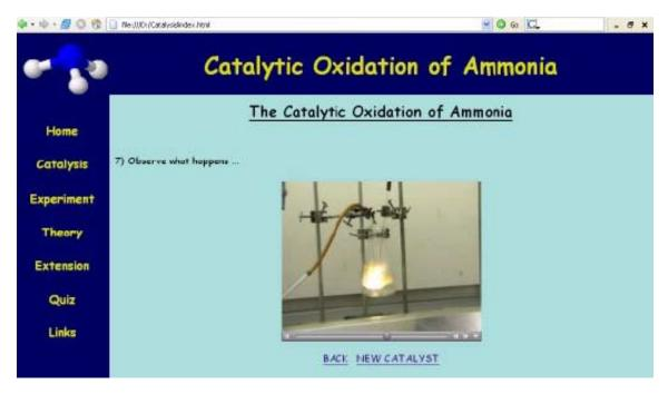
Once the reaction had started, the platinum continued to glow without further heating. Brown fumes of nitrogen dioxide appeared in the flask. In order to show that the platinum was the catalyst, two other metals were used; copper and constantan. The results showed that neither of these metals would catalyse the process.
