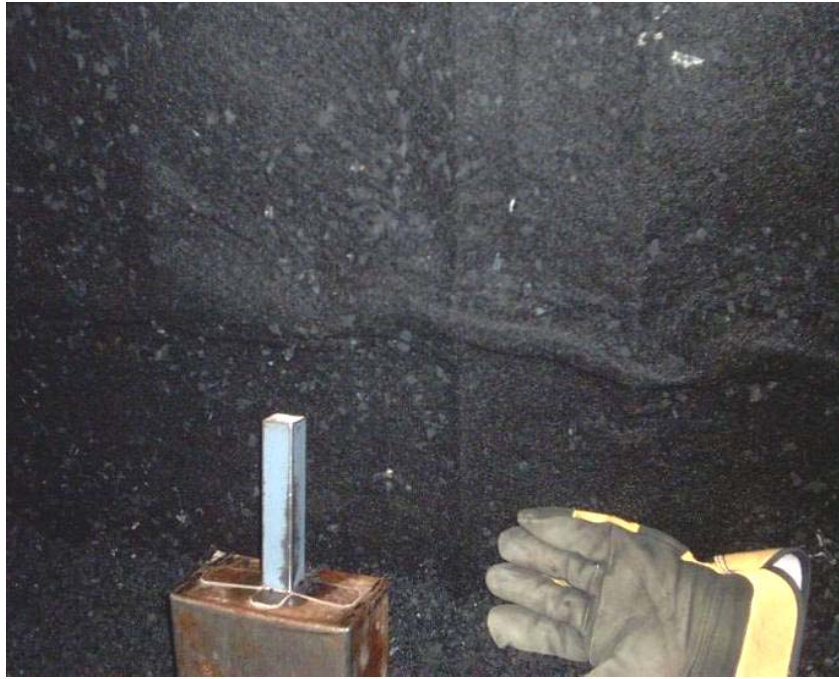
Figure 4.26 Folding of the geotextile approximately 500 mm above the base of the sample in test with fusion welded seam.
