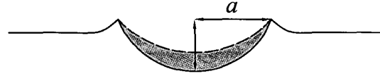
Fig. 8. The indentation in an isotropic semi-infinite body, produced by a spherical indenter, after [12].
